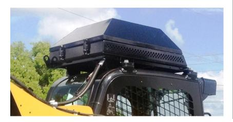
Supertrak is proud to offer an Industry leading reversible fan driven Hydraulic Cooler Kits for your Caterpillar® C / D Series SSL, MTL, CTL's models. This kit mounts to the standard cab and is field installed to supply additional cooling for the Machines hyd system. Standard equipped with an auto reversing fan, debris protected guarding, high pressure hoses.
